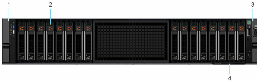
Figure 2. Front view of 16 x 2.5-inch drive system
