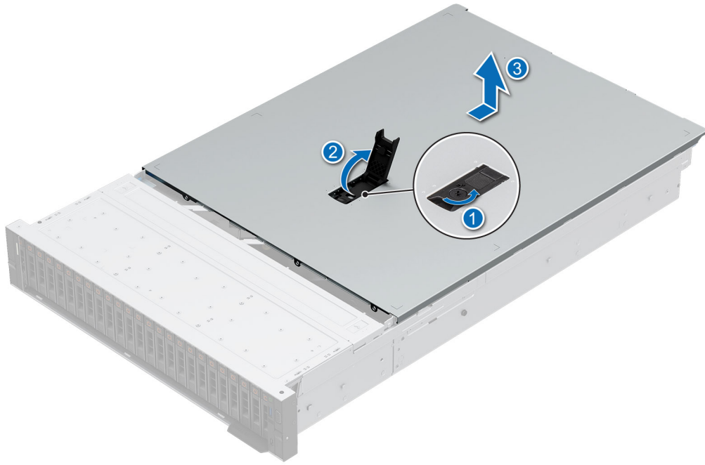
Figure 27. Removing the system cover
