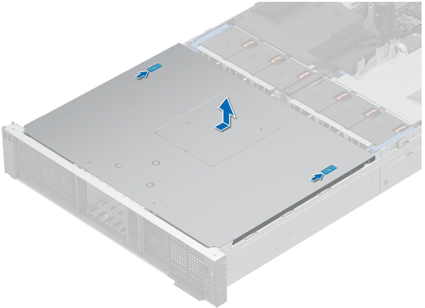
Figure 26. Removing the drive backplane cover
