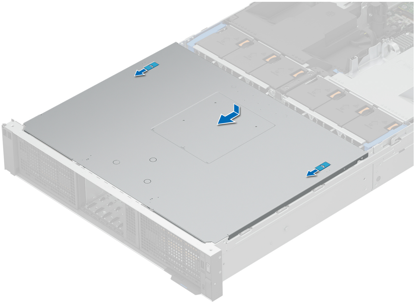
Figure 27. Installing the drive backplane cover
