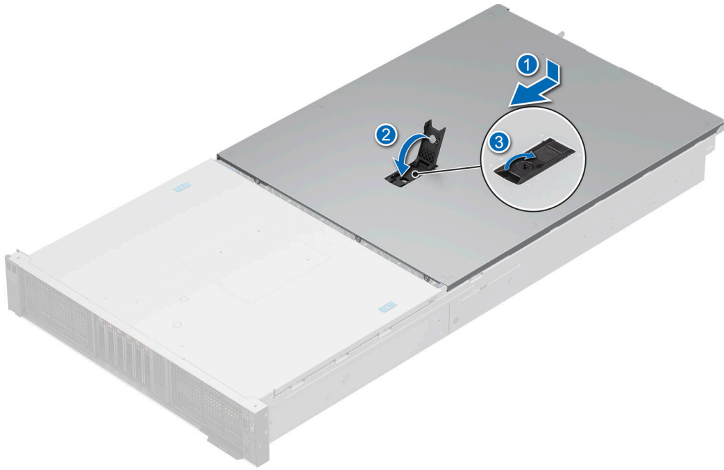
Figure 25. Installing the system cover
