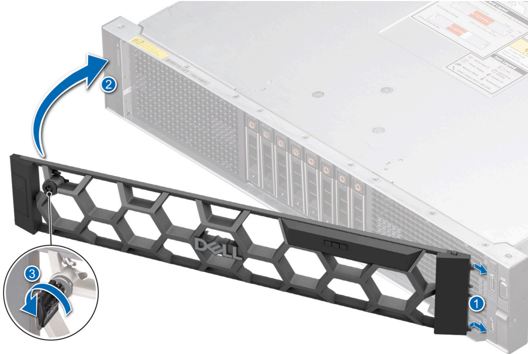
Figure 23. Installing the front bezel
