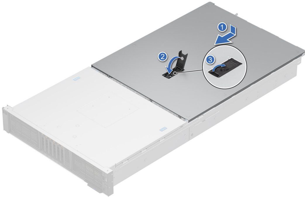
Figure 25. Installing the system cover
