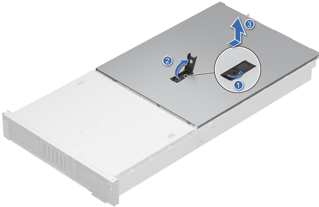
Figure 24. Removing the system cover
