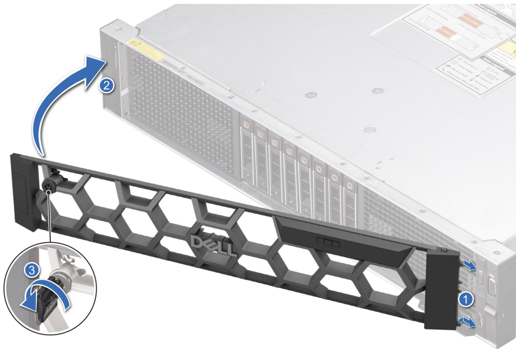
Figure 23. Installing the front bezel
