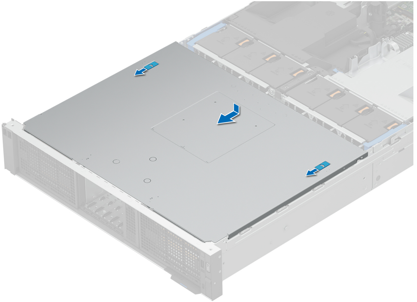
Figure 27. Installing the drive backplane cover
