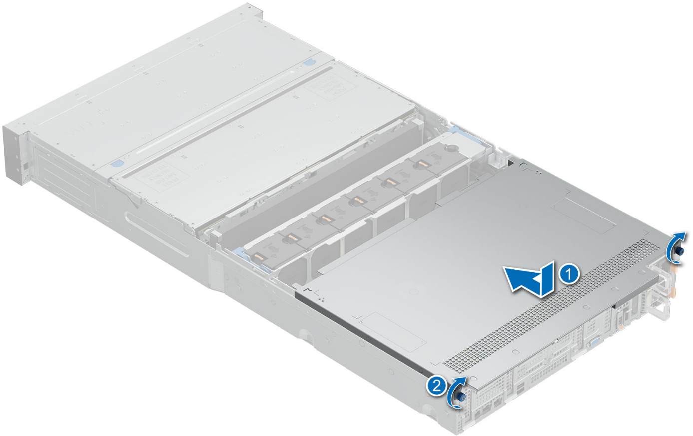
Figure 40. Installing rear system cover
