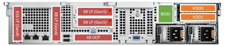
Figure 14. Rear view of the system with Riser 1d
