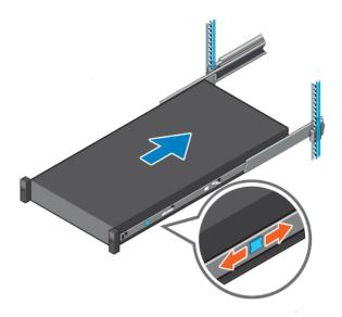
Figure 30. Slide system into the rack
