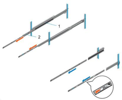
Figure 31. Pull out the intermediate rail
