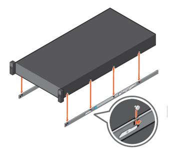
Figure 32. Attach the inner rails to the system
