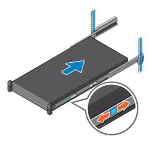
Figure 34. Slide system into the rack
