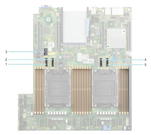
Figure 21. Expansion card slot connectors
