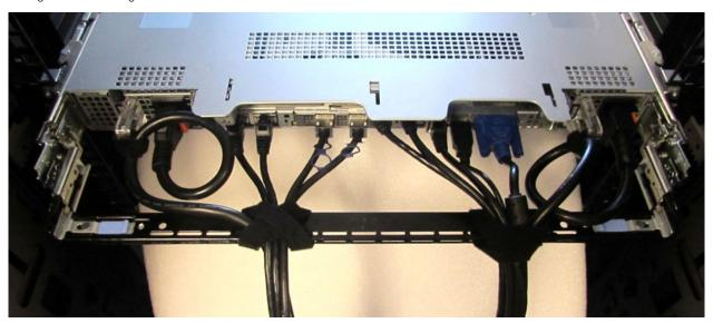
Figure 27. Cabled strain relief bar
