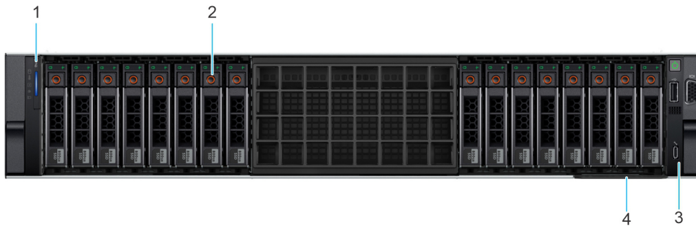
Figure 2. Front view of 16 x 2.5-inch drive system
