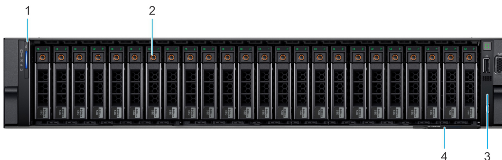
Figure 1. Front view of 24 x 2.5-inch drive system
