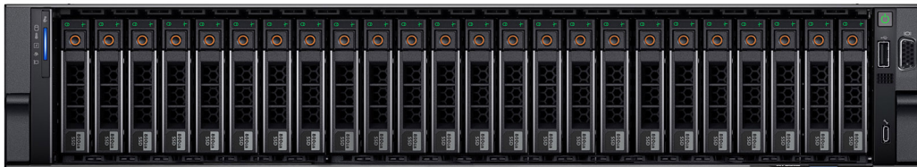
Figure 1. Front view of 24 x 2.5-inch drive system
