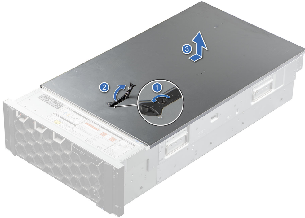
Figure 36. Removing the system cover
