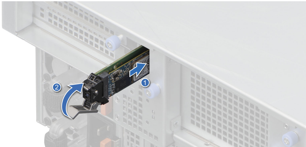
Figure 186. Installing the BOSS-N1 card carrier
