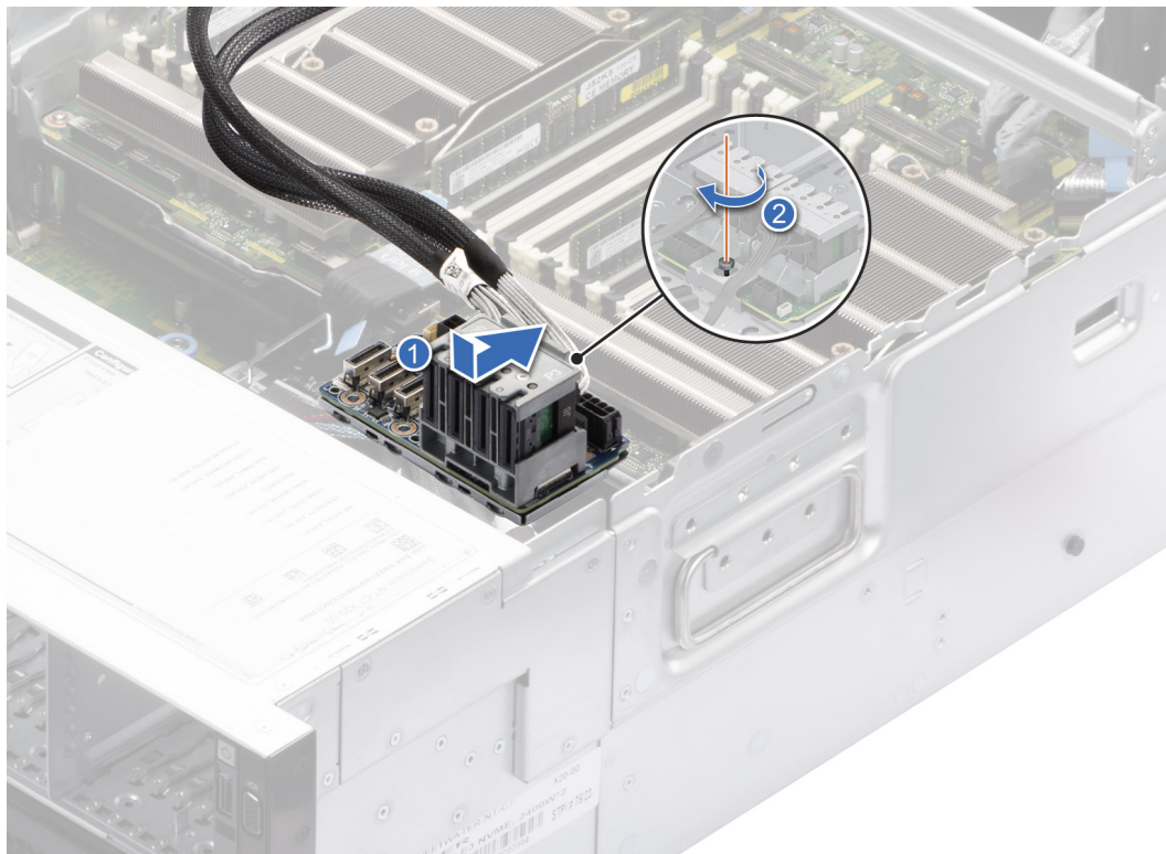
Figure 94. Installing the EDSFF E3.S backplane module
