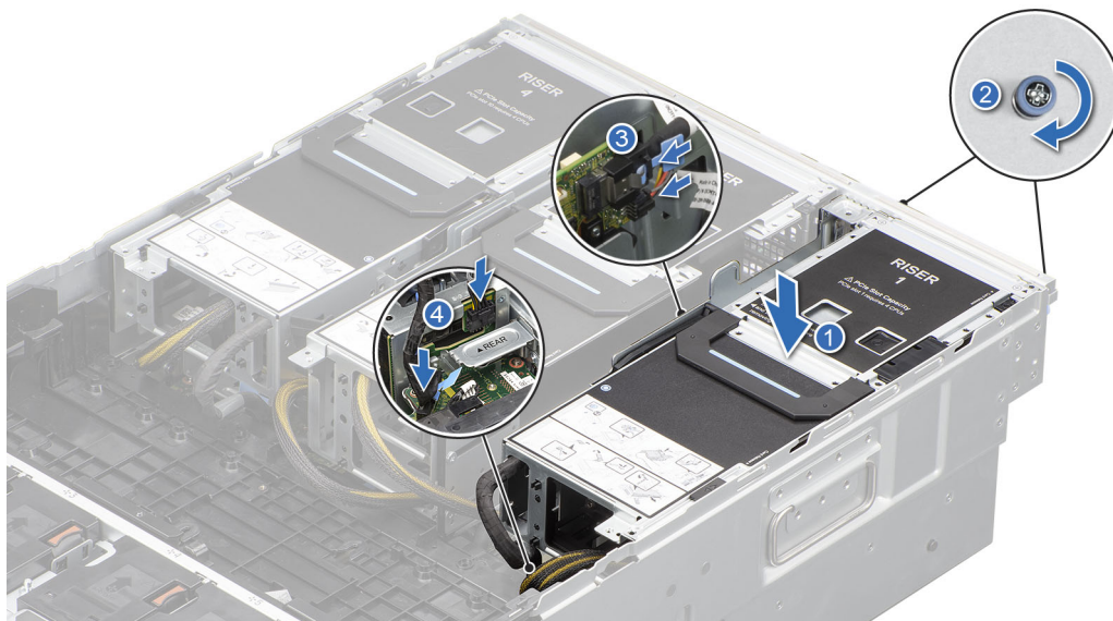
Figure 132. Installing the expansion card riser 1
