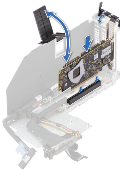
Figure 127. Installing an expansion card into the expansion card riser
