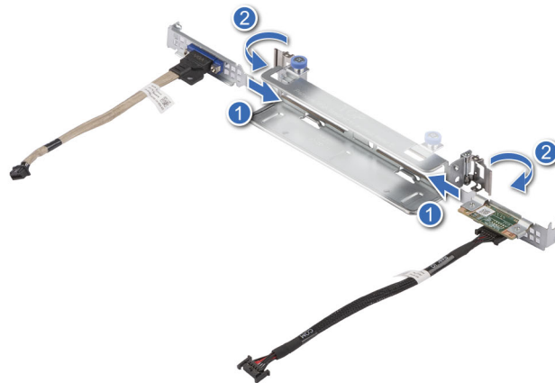
Figure 173. Installing the VGA and Serial COM port
