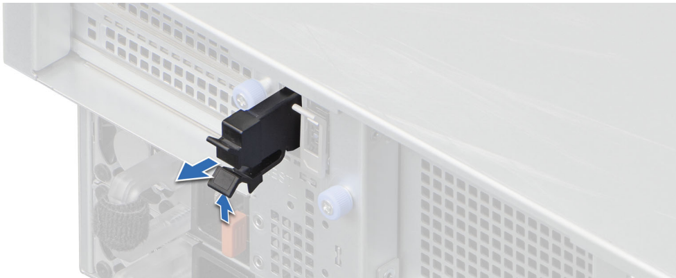
Figure 177. Removing the BOSS-N1 card carrier blank
