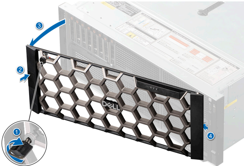
Figure 30. Removing the front bezel with the LCD panel
