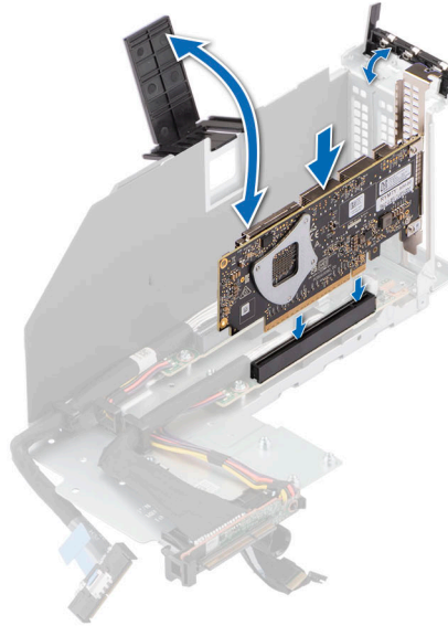
Figure 123. Installing an expansion card into the expansion card riser
