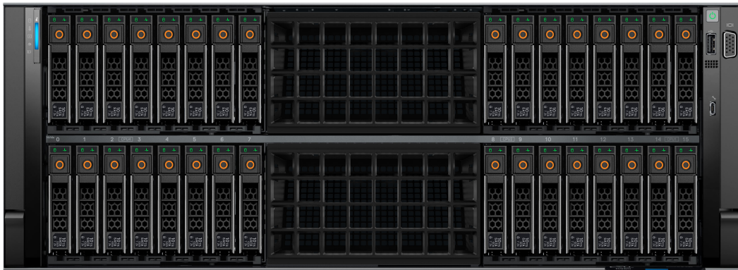
Figure 1. Front view of 32 x 2.5-inch drive system
