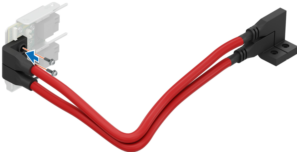
Figure 50. Connect the left midplane power cables to the midplane
