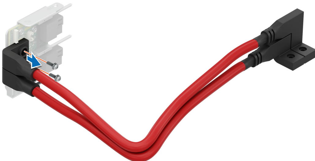
Figure 49. Removing the left midplane power cables
