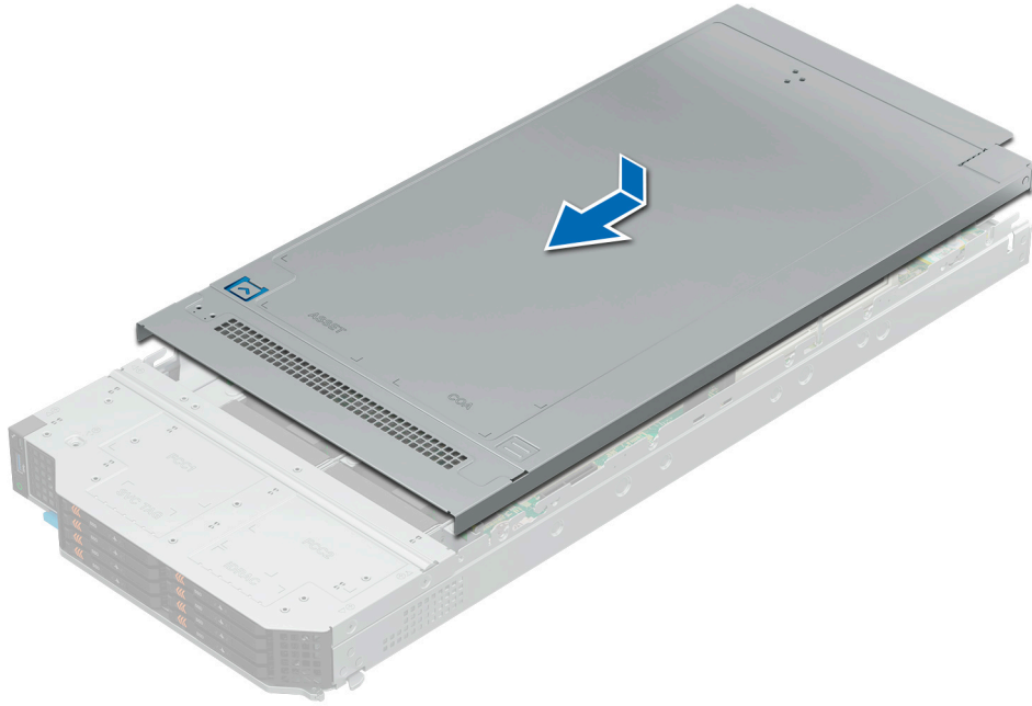
Figure 23. Installing the sled cover
