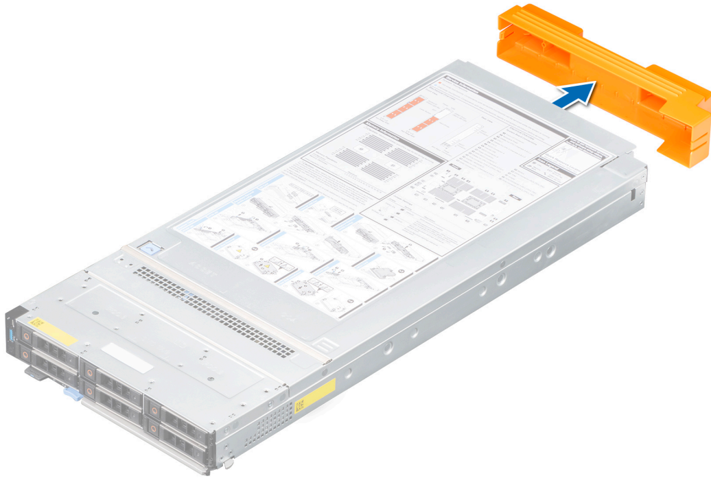
Figure 20. Removing the I/O connector cover from sled
