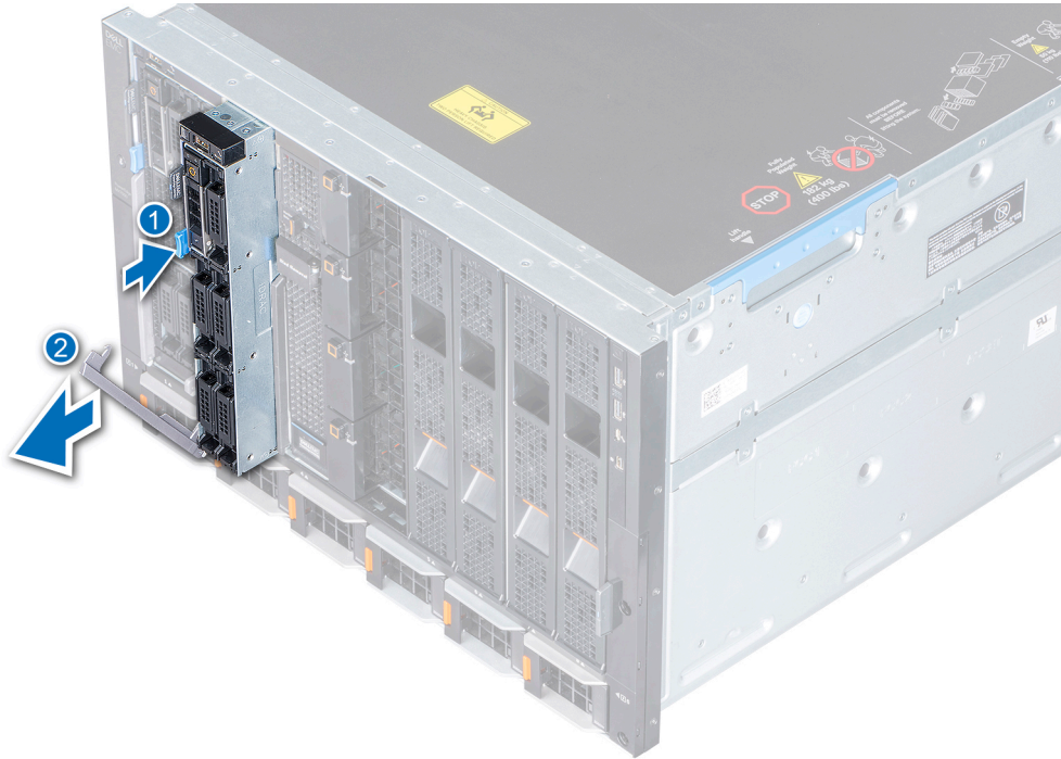
Figure 18. Removing the sled from enclosure
