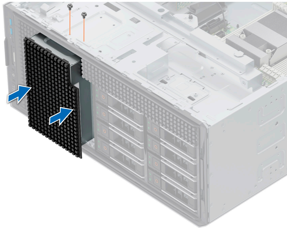
Figure 118. Installing the NVMe drive bay blank
