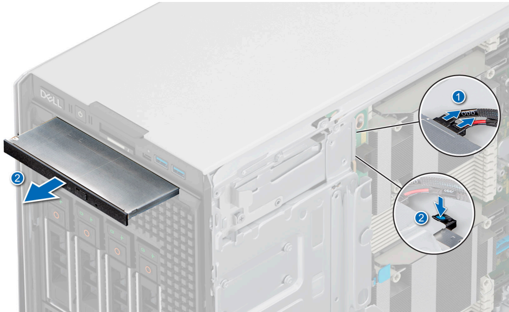
Figure 127. Removing the optical drive
