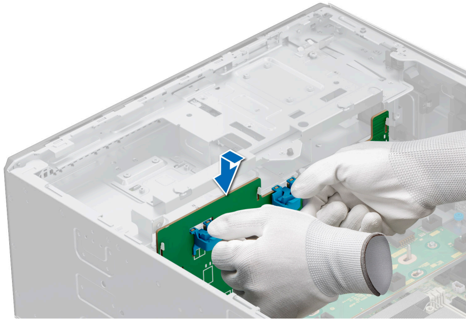
Figure 110. Installing the 3.5-inch drive backplane
