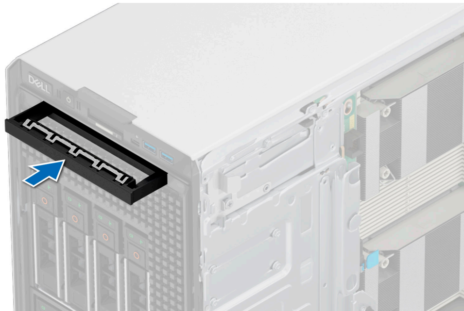
Figure 126. Installing the optical drive blank
