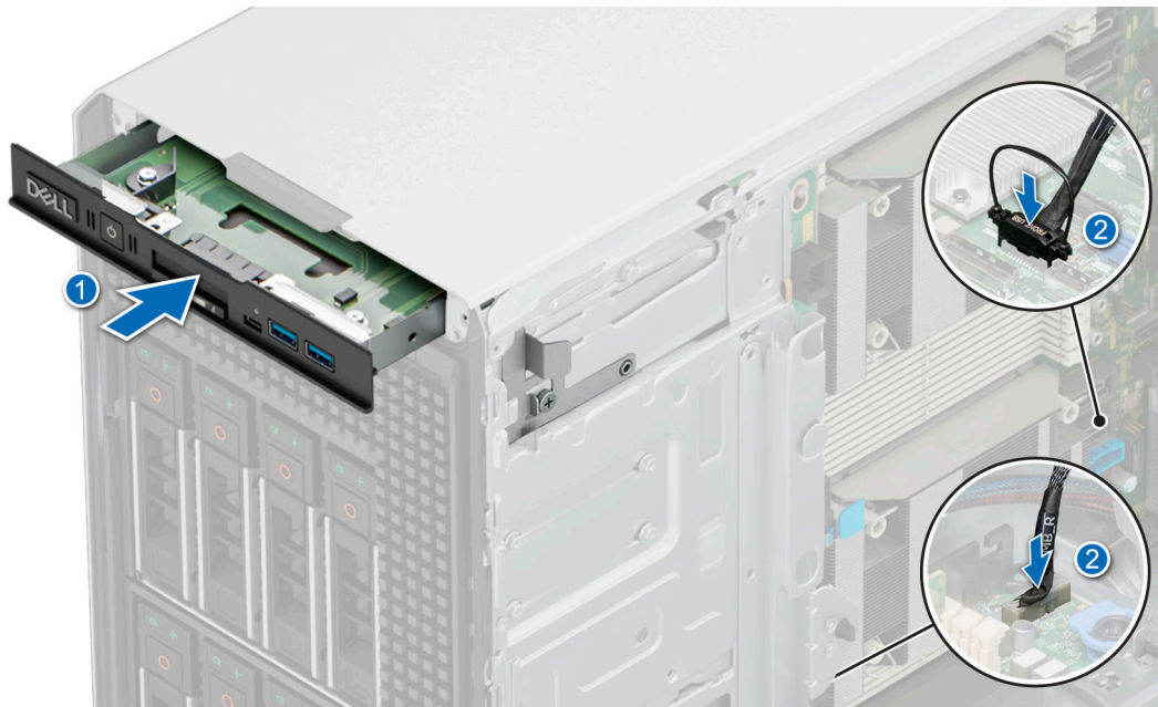
Figure 134. Installing the front IO module
