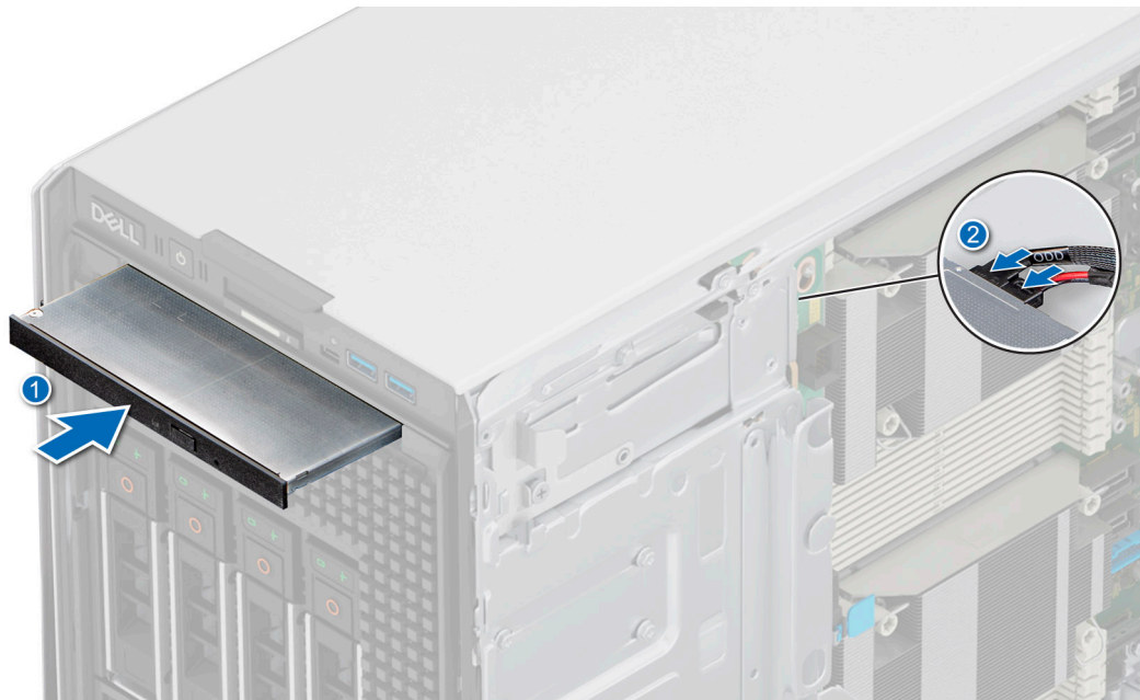
Figure 128. Installing the optical drive
