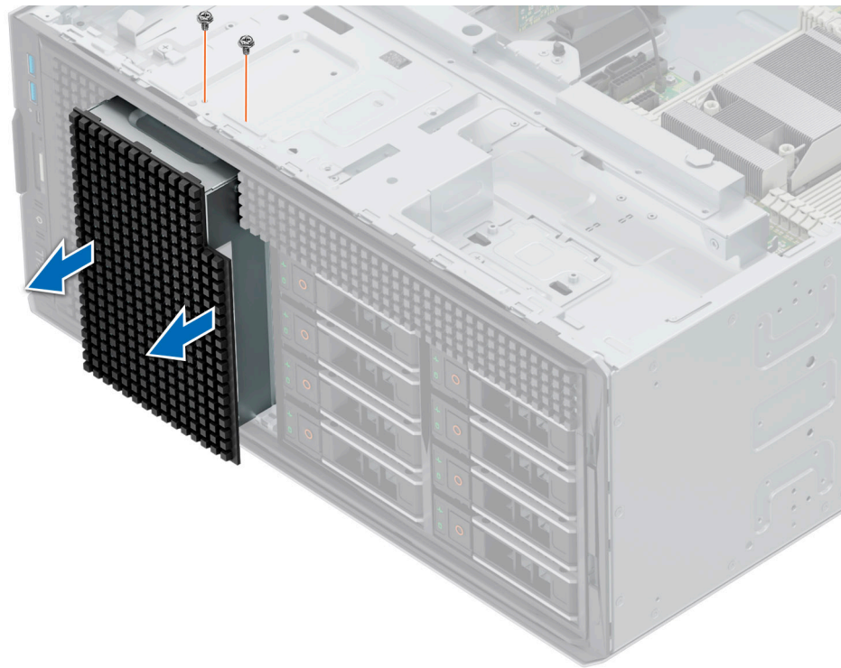
Figure 115. Removing the NVMe drive bay blank
