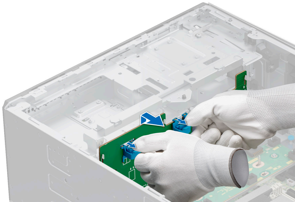
Figure 109. Removing the 3.5-inch drive backplane
