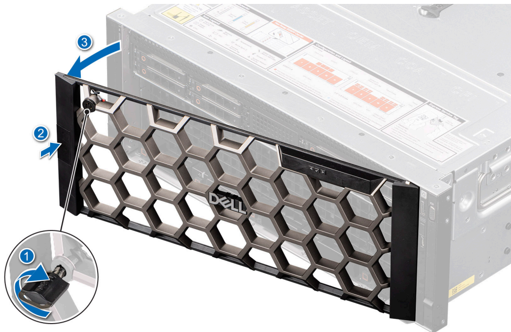
Figure 16. Removing the front bezel with the LCD panel
