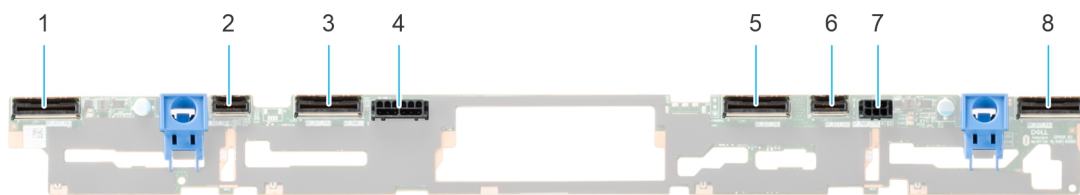
Figure 38. 8 x 2.5-inch NVMe drive backplane
