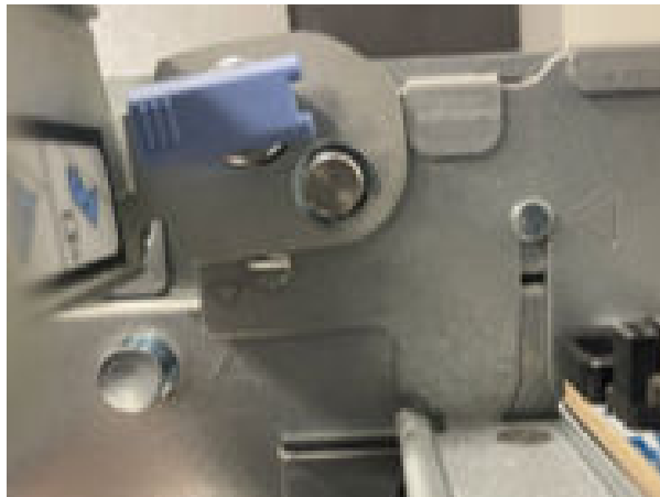
Figure 143. Alignment of the triangle mark inside and outside the chassis
