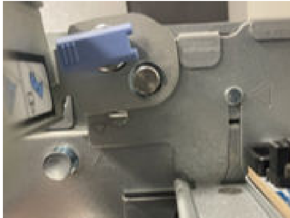
Figure 151. Alignment of the triangle mark inside and outside the chassis
