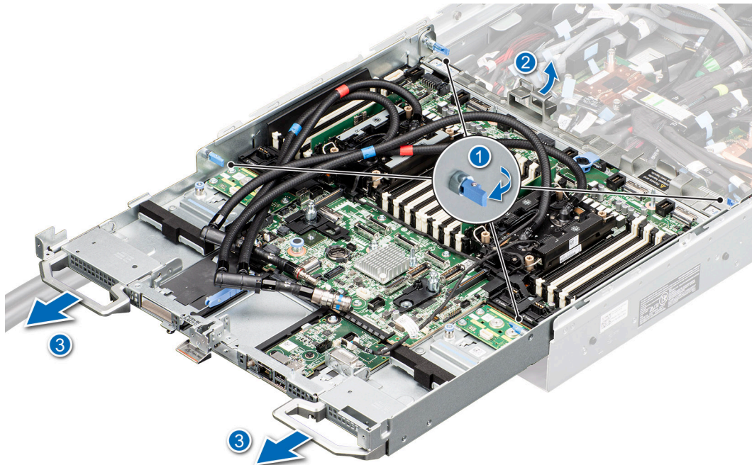
Figure 148. Sliding out the system board tray
