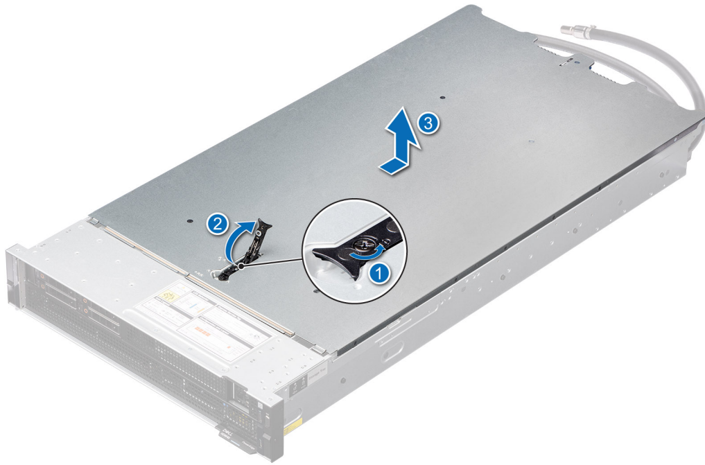
Figure 20. Removing the system cover
