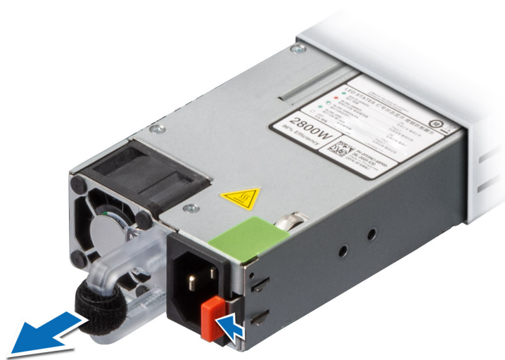
Figure 87. Removing a power supply unit
