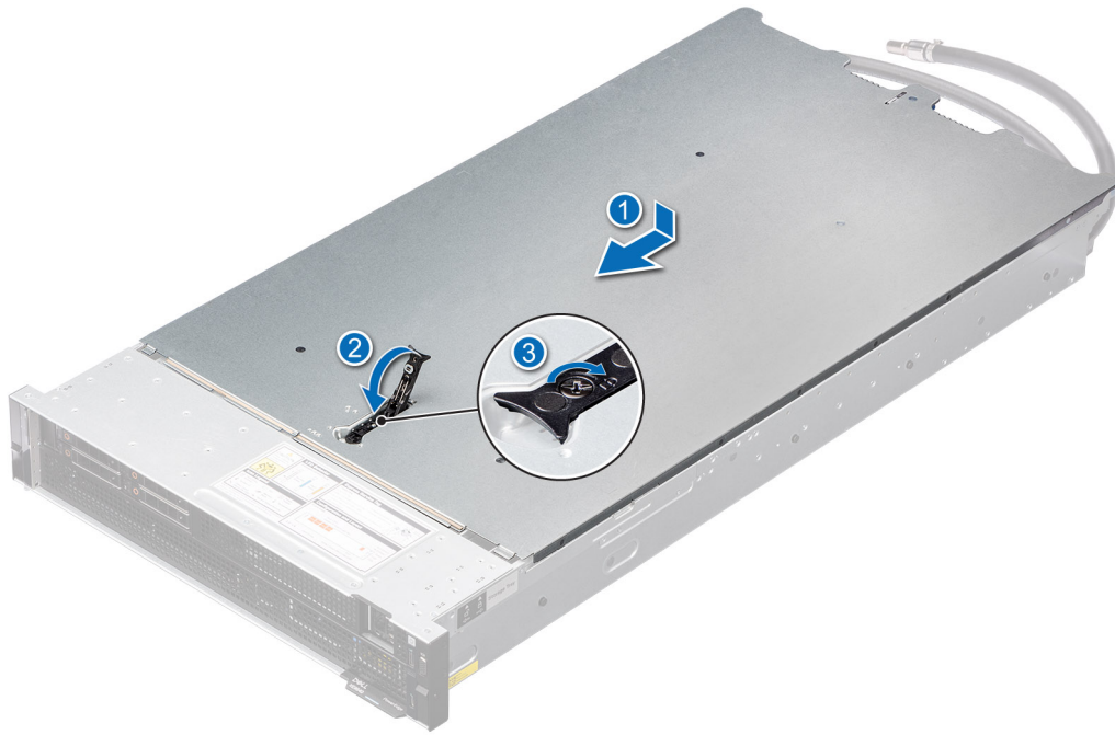
Figure 21. Installing the system cover
