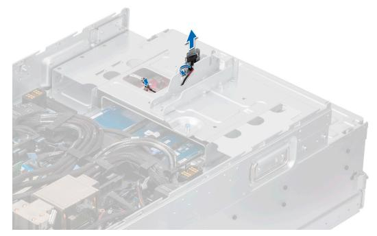
Figure 89. Removing the intrusion switch module
