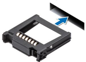
Figure 41. Installing a drive blank
