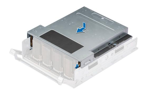
Figure 127. Installing the H100 GPU top cover
