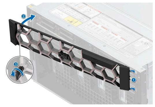
Figure 27. Installing the front bezel with the LCD panel
