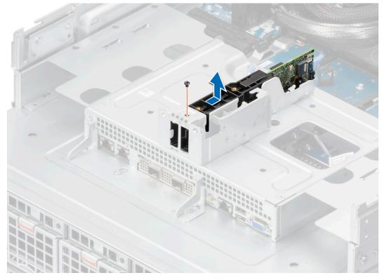
Figure 94. Removing the BOSS-N1 module
