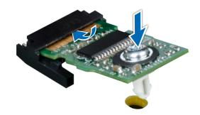
Figure 161. Installing the TPM
