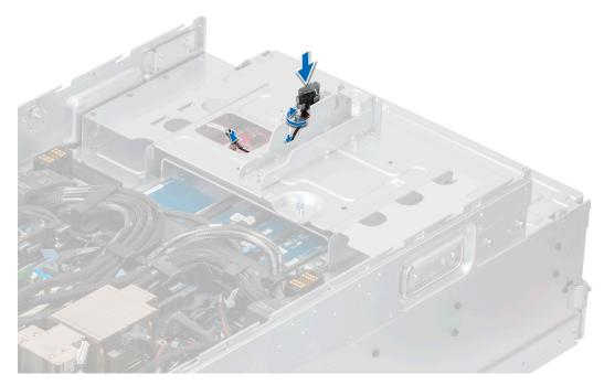
Figure 90. Installing the intrusion switch module
