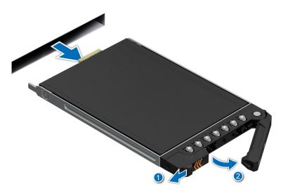
Figure 48. Removing an EDSFF E3.S drive carrier
