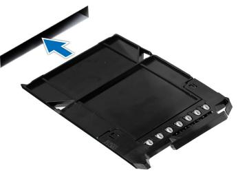
Figure 47. Installing an EDSFF E3.S drive blank
