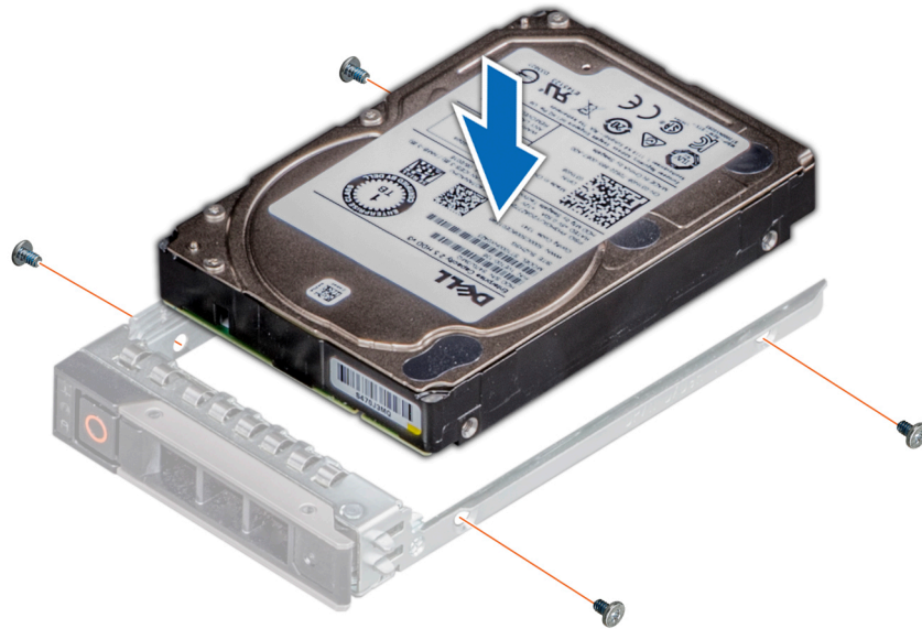
Figure 59. Installing a drive into the drive carrier
