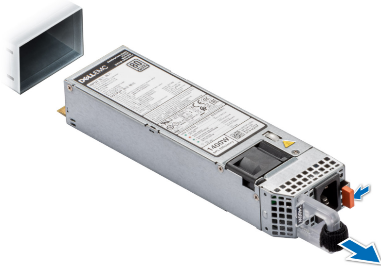
Figure 114. Removing a power supply unit from Rear Accessed configuration
