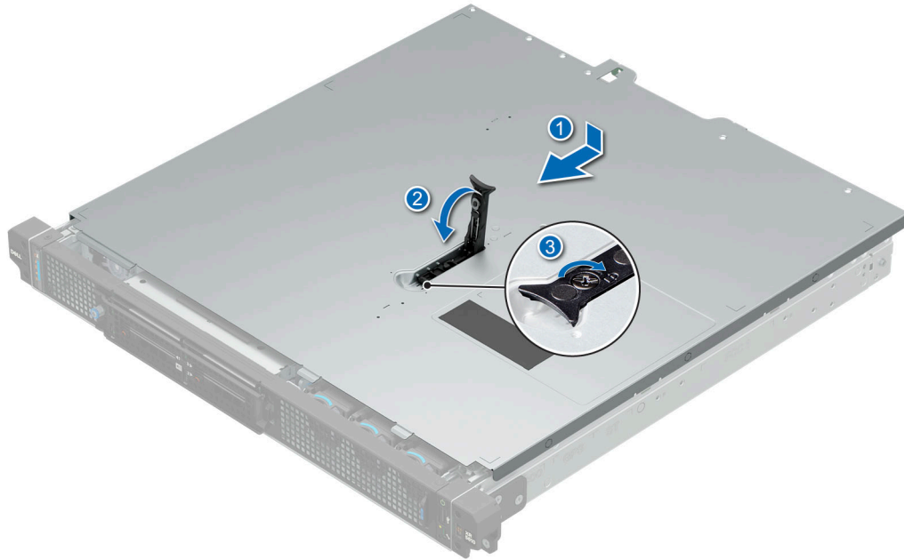
Figure 37. Installing the system cover for Rear Accessed configuration
