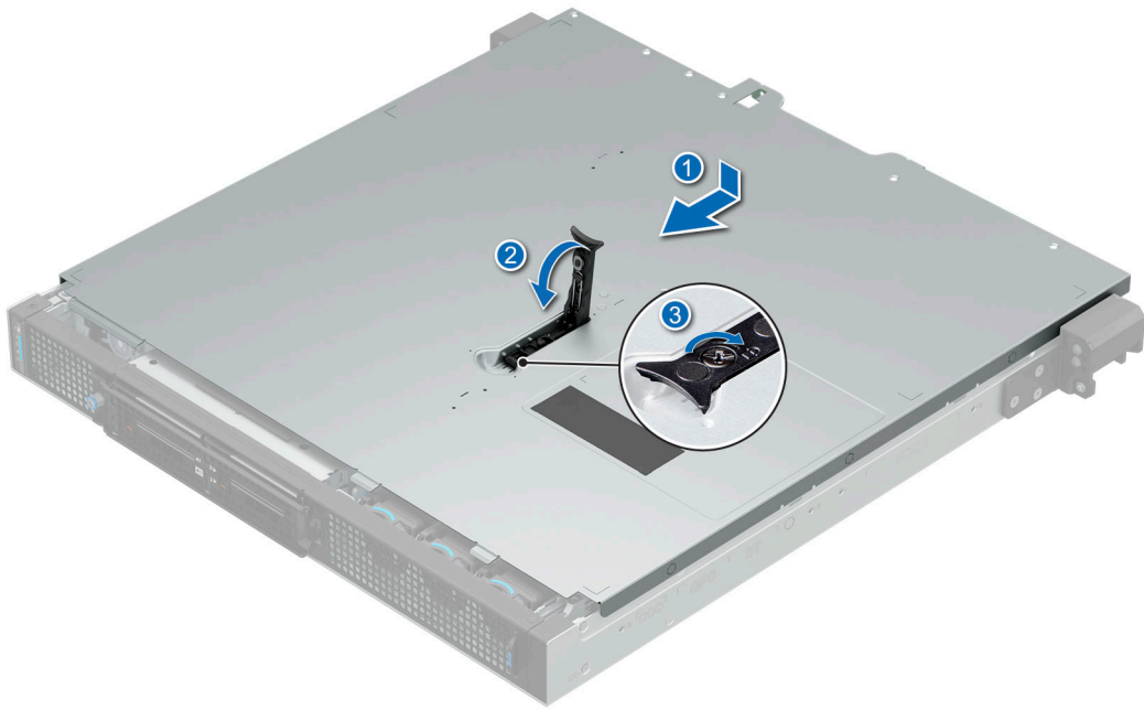
Figure 38. Installing the system cover for Front Accessed configuration
