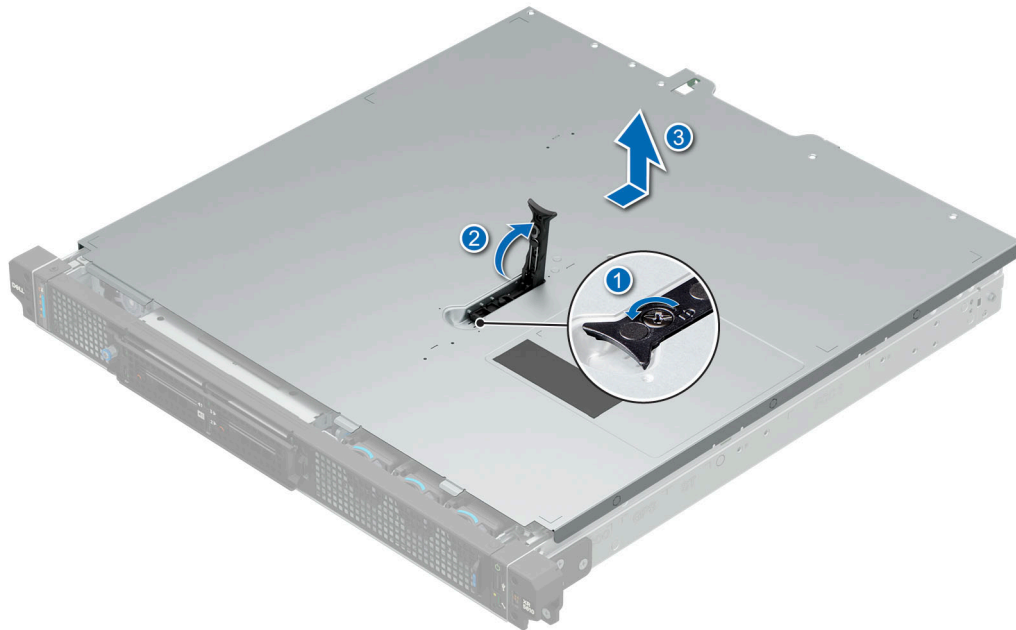
Figure 35. Removing the system cover for Rear Accessed configuration
