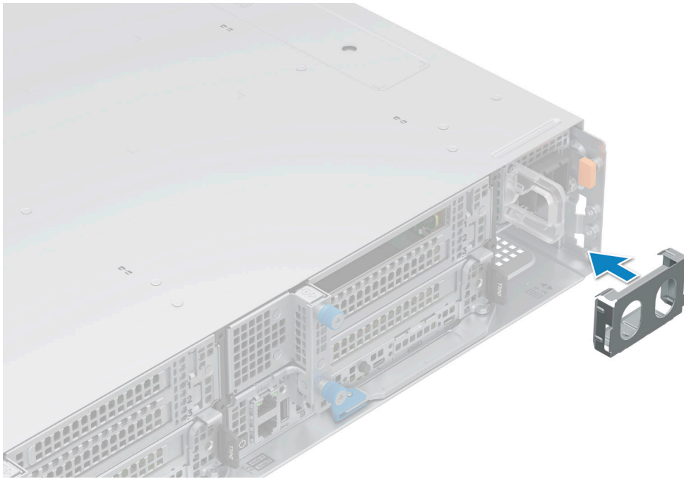
Figure 22. Installing a power supply unit blank
