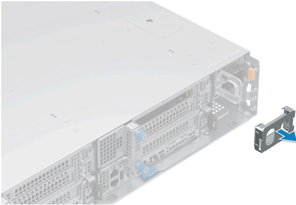
Figure 19. Removing a power supply unit blank
