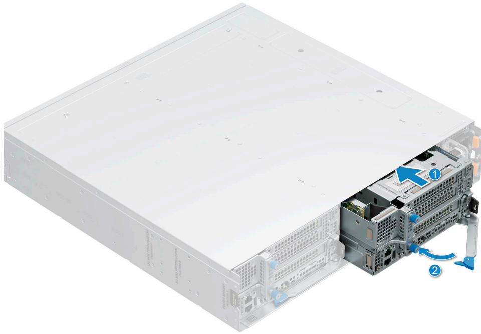
Figure 14. Installing a sled into XR8000r
