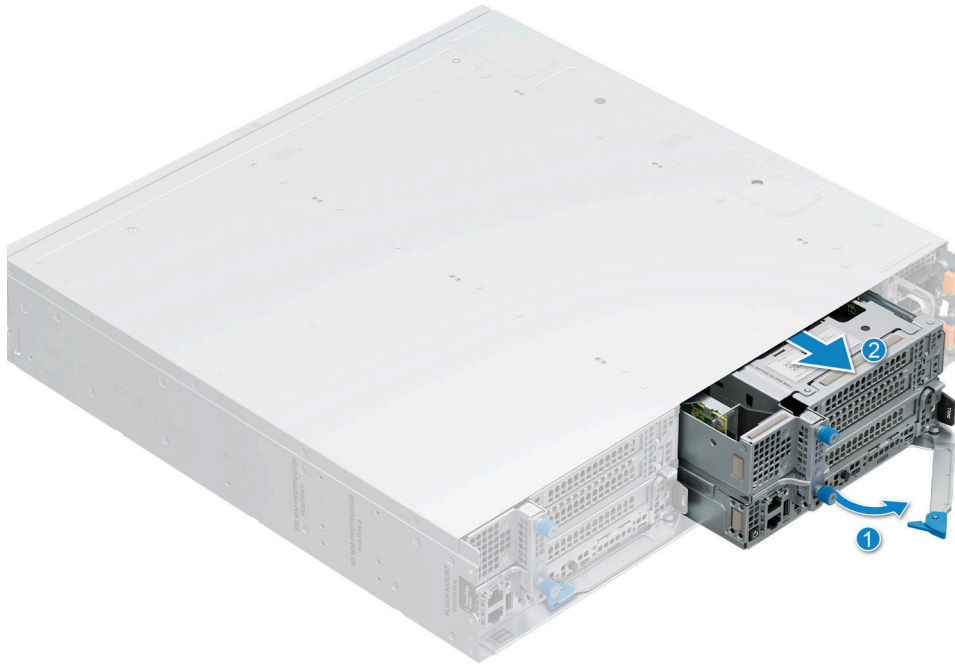
Figure 13. Removing a sled from XR8000r
