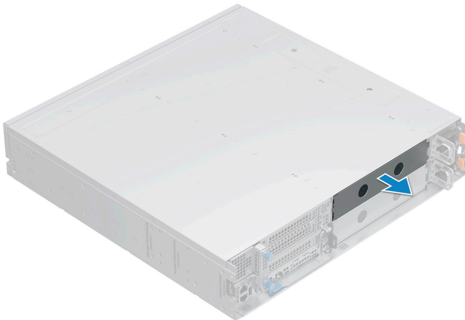
Figure 11. Removing a sled blank
