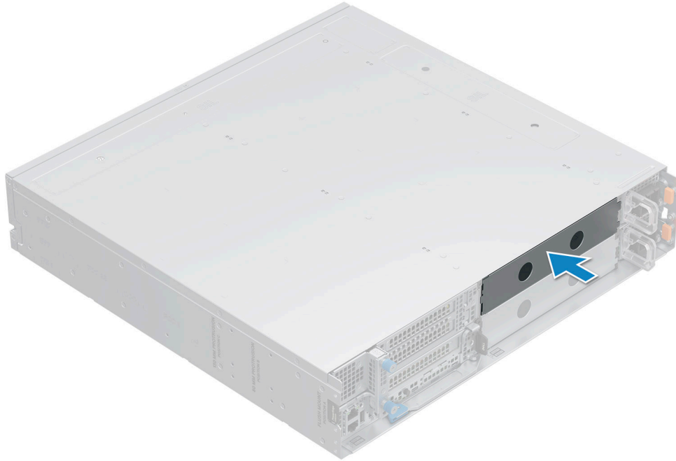
Figure 12. Installing a sled blank
