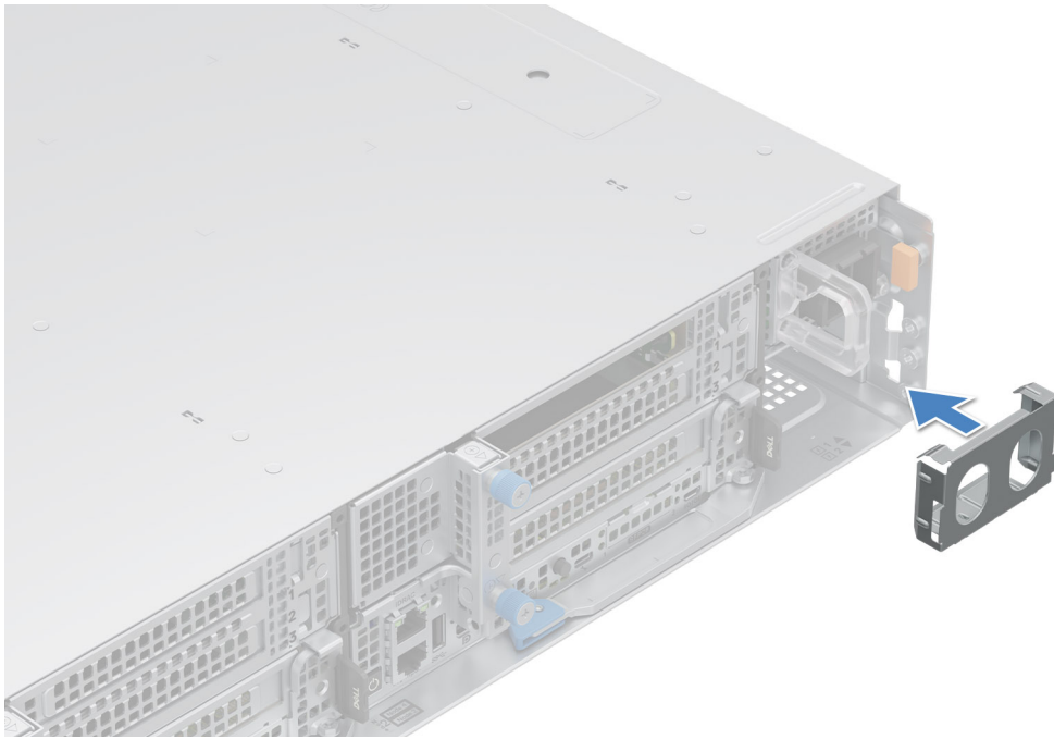
Figure 22. Installing a power supply unit blank
