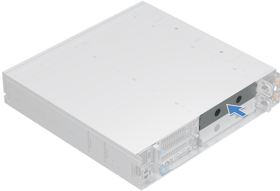
Figure 12. Installing a sled blank
