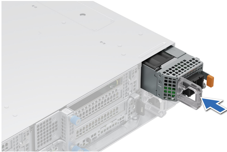
Figure 21. Installing a reverse air flow (RAF) power supply unit
