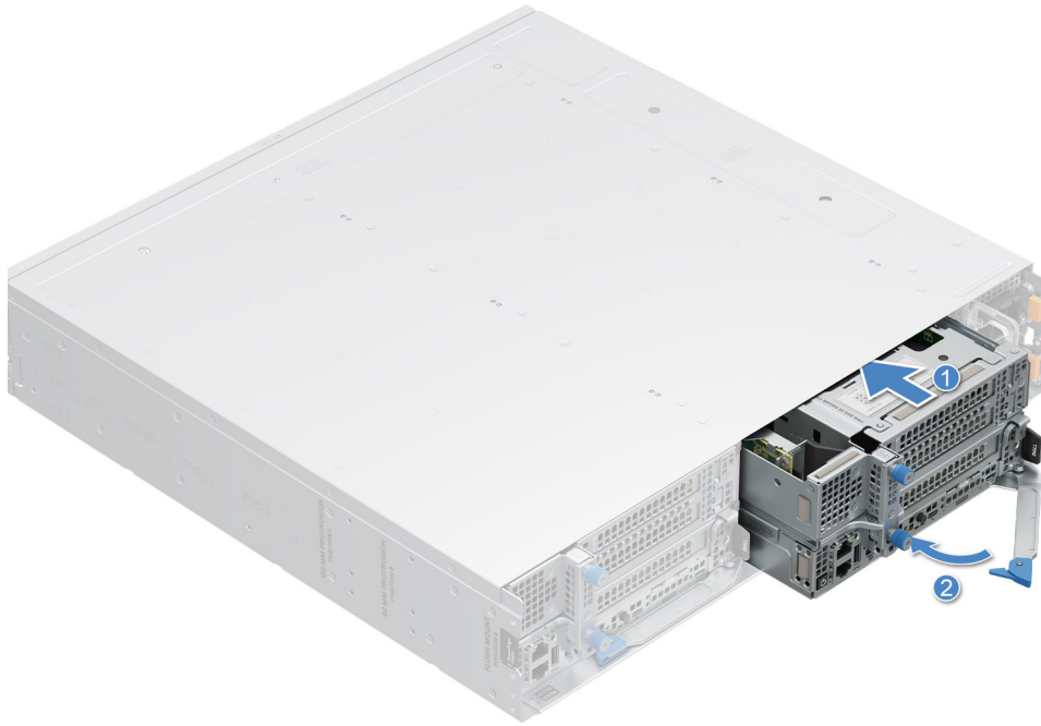
Figure 14. Installing a sled into XR8000r
