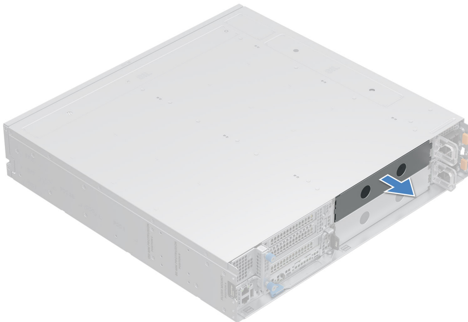
Figure 11. Removing a sled blank
