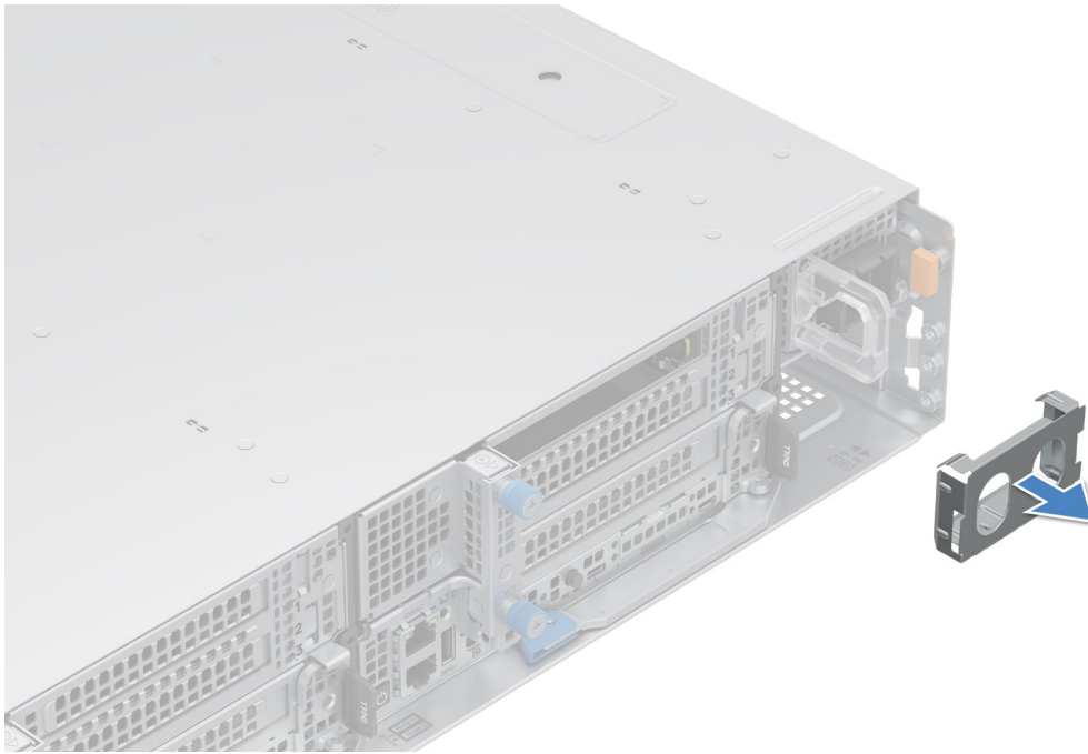
Figure 19. Removing a power supply unit blank
