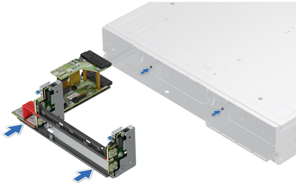
Figure 18. Installing the power module assembly
