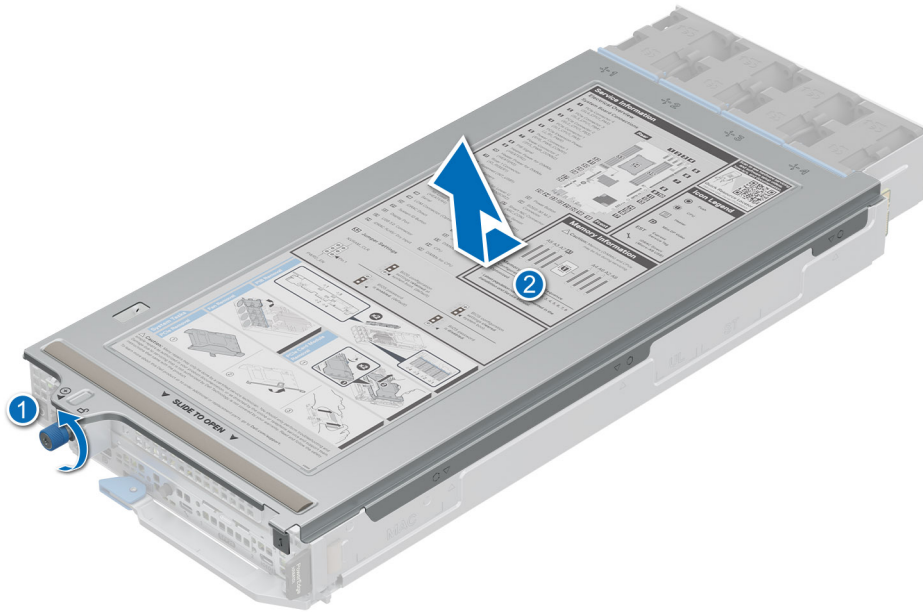
Figure 19. Removing the sled cover
