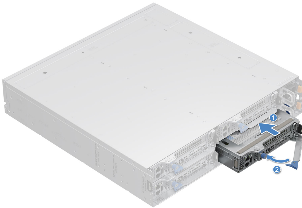
Figure 18. Installing a sled into XR8000r
