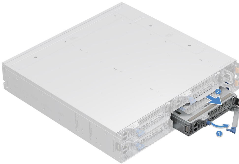
Figure 17. Removing a sled from XR8000r
