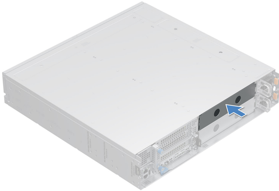
Figure 16. Installing a sled blank
