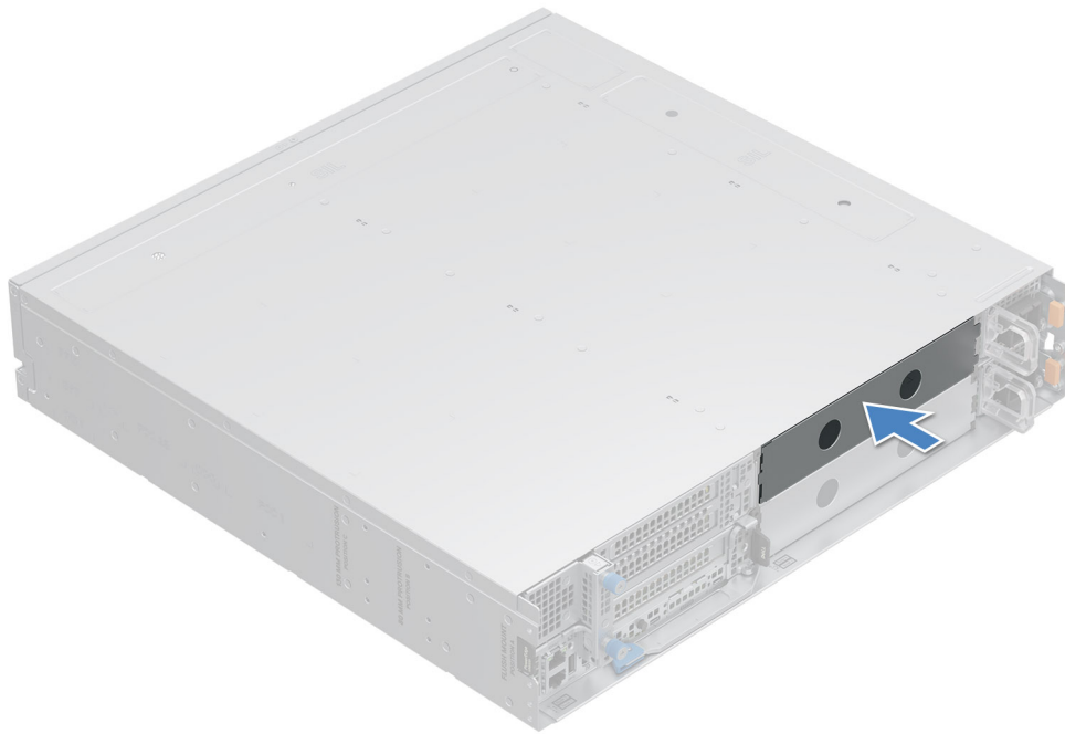
Figure 16. Installing a sled blank
