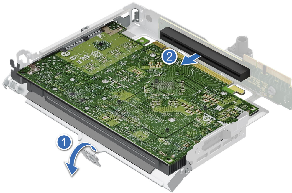
Figure 61. Removing the Nokia Cloud RAN SmartNIC 2x QSFP56-DD from the Riser 2
