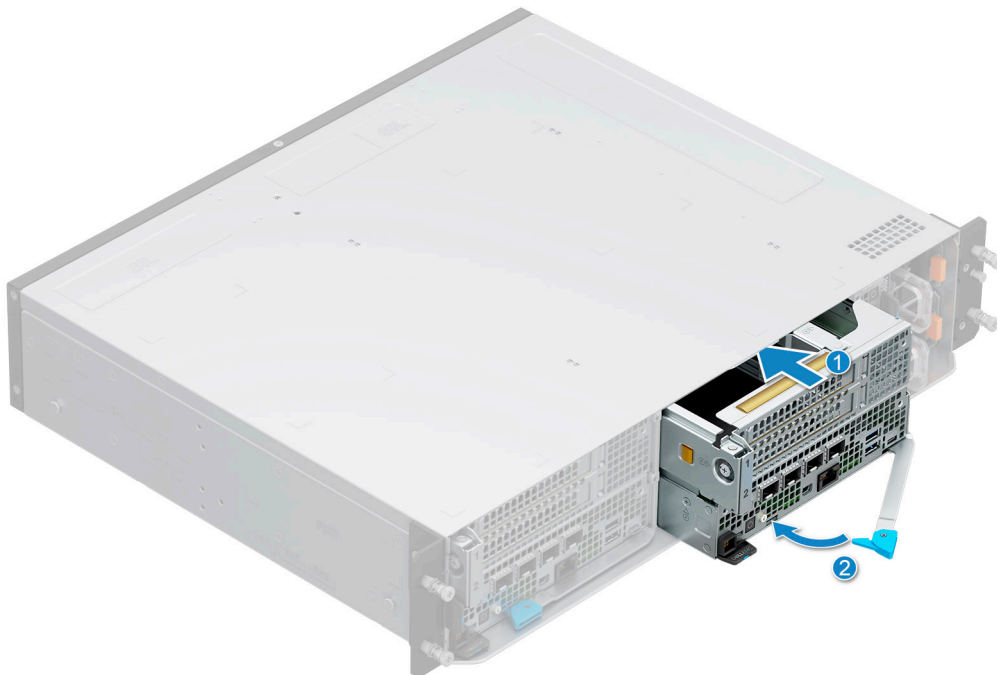
Figure 21. Installing a 2U sled into XR4000r
