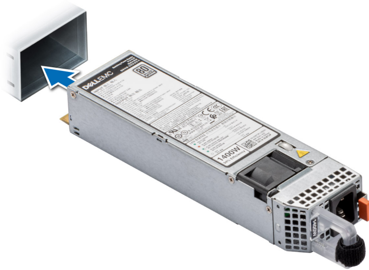
Figure 31. Installing a normal air flow (NAF) power supply unit
