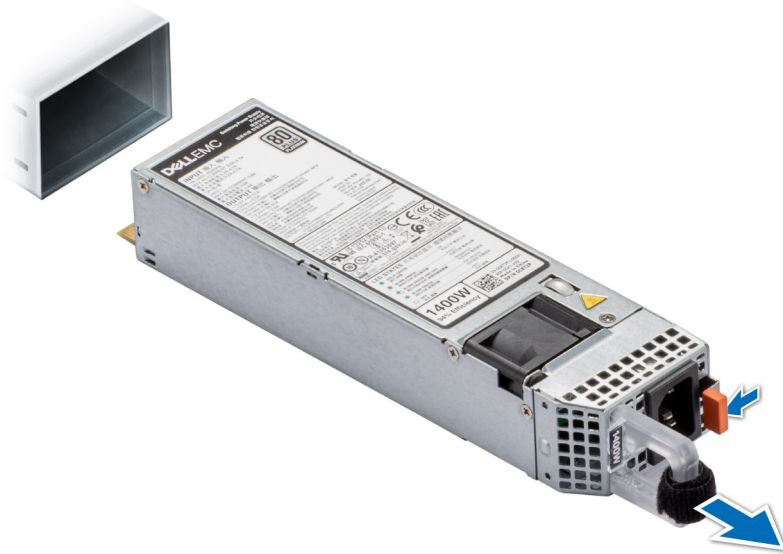
Figure 29. Removing a normal air flow (NAF) power supply unit
