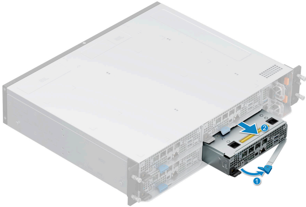
Figure 18. Removing a 1U sled from XR4000r
