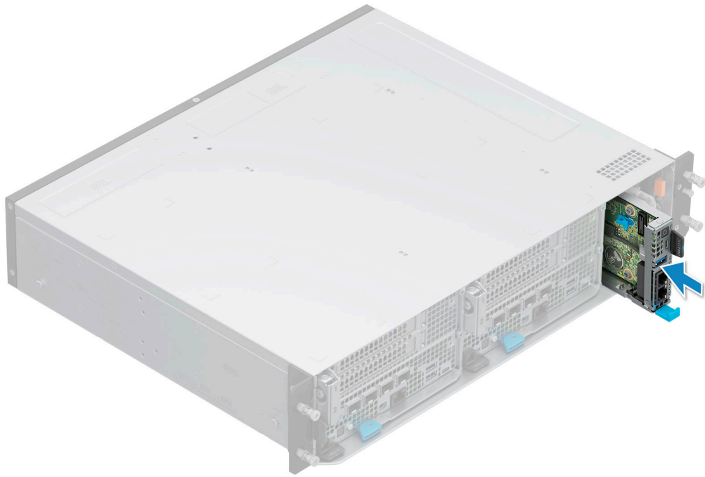
Figure 37. Installing the witness sled
