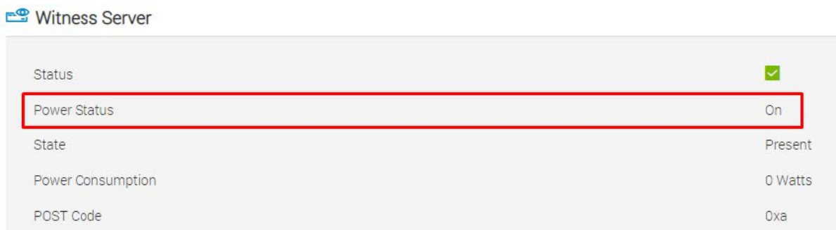
Figure 20. iDRAC GUI Witness power status
