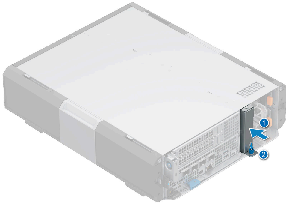
Figure 42. Installing the witness sled blank on XR4000z
