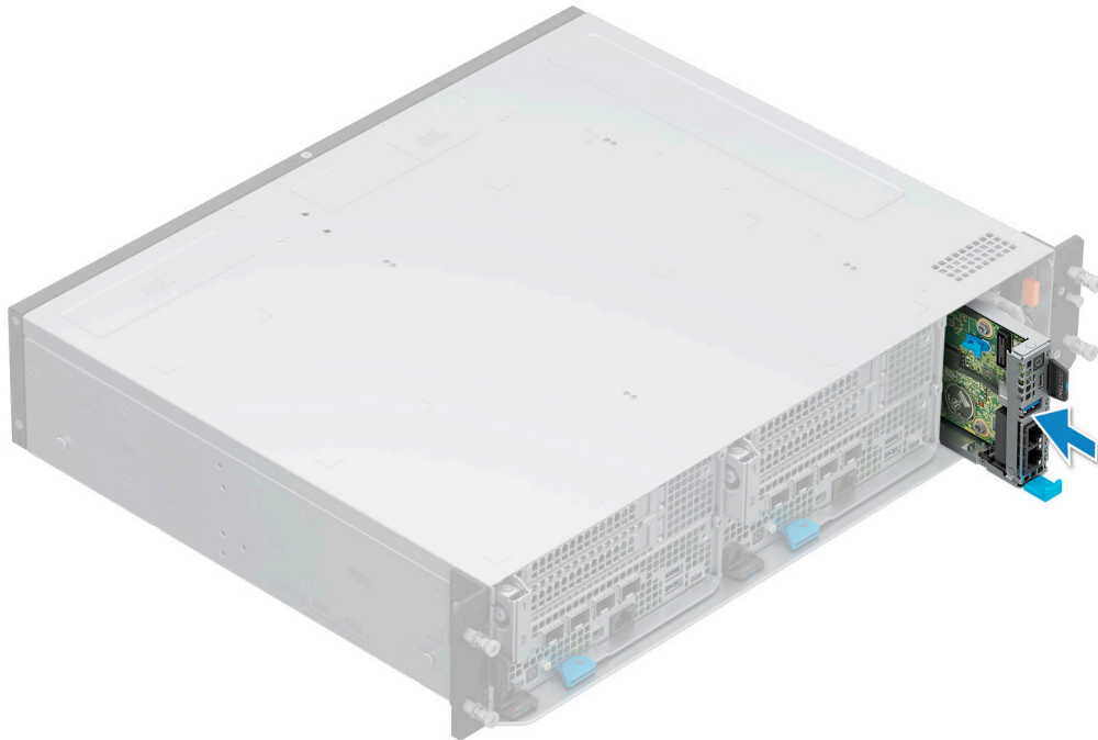
Figure 39. Installing the witness sled into XR4000r
