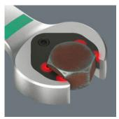
The Joker's clever double-hex geometry delivers a very positive connection with nuts or bolts - it's a perfect fit. Serated teeth on the hardened metal plate provide grip in the Joker's open end literally bite themselves into the bolt, with its extremely hard tips. Both features combine to prevent slipping, even at higher torque.
