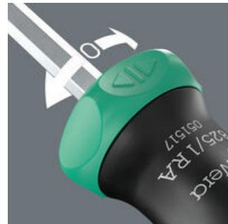
Intuitive switching of the ratchet mechanism. Turn the switch clockwise for clockwise screwdriving; turn it counterclockwise for counterclockwise screwdriving. Use position 0 to deactivate the ratchet mechanism for precise working.
