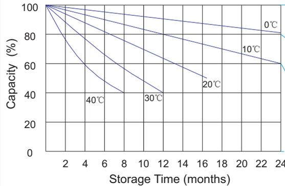
Supplementary charge required before use. (Carry out supplementary charge before use if 100% capacity is required)
