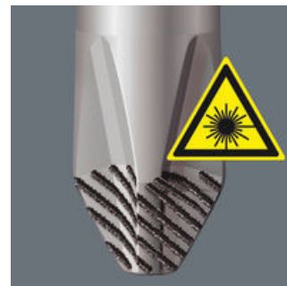
A precisely-focused laser creates a sharp-edged surface structure. Wera Lasertip "bites" itself into the screw head and prevents any slips out of the recess. It is available for screwdrivers for slotted, Phillips and Pozidriv screws.
