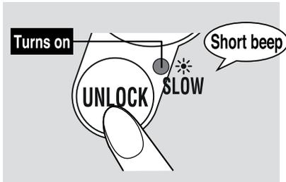
The **UNLOCK** light turns on and hot water can be dispensed.
