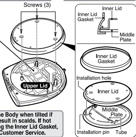
Hot water may leak from the gap between the Upper Lid and the Body when tilted if the Inner Lid Gasket becomes old and turns white. This may result in scalds. If hot water spews from the gap or there is steam even after replacing the Inner Lid Gasket, other parts may be in need of repair. Please contact Zojirushi Customer Service.
