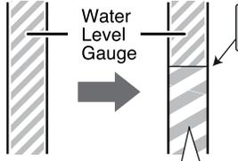
The stripes on the Water Level Gauge appear thicker when water is added.
