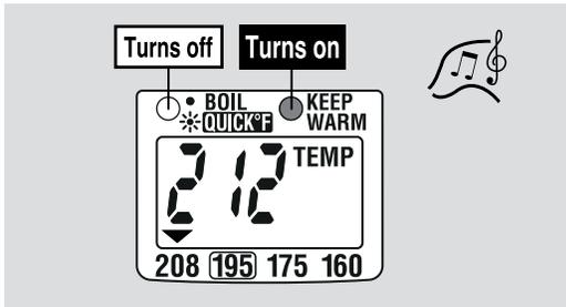
When the boiling process has completed, a melody sounds, the BOIL light turns off and the KEEP WARM light turns on.
