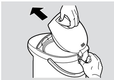
**2** Hold the product with both hands and dispose water where indicated "EMPTY FROM HERE" on the wall of the Inner Container.
