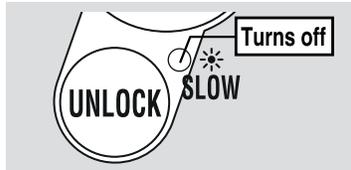
10 seconds after dispensing, the UNLOCK light turns off and the Automatic Dispense Lock is activated.
