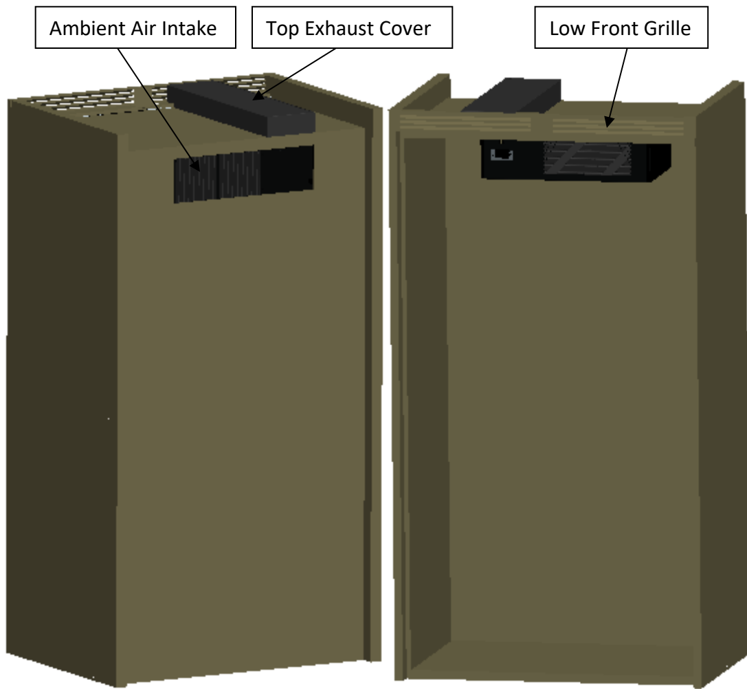
Fig. 2.9 Cooling Unit Installed (Low Front Grille)
