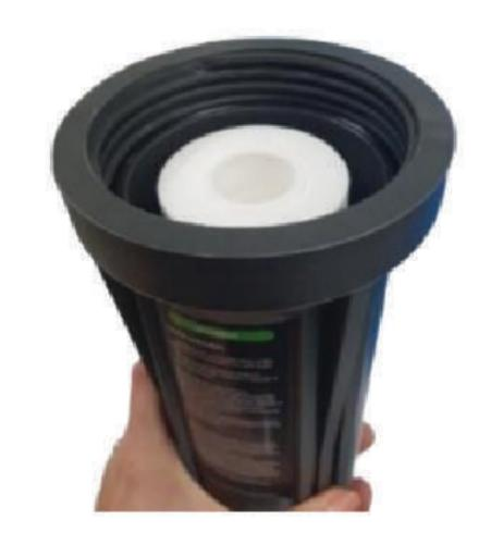
7. CHECK O-RING & FILTER - Lubricate the o-rings with food grade silicone lubricant or similar if needed. Replace O-ring if kinked or damaged. It is very important the filter and O'Ring are seated properly in the housing.
