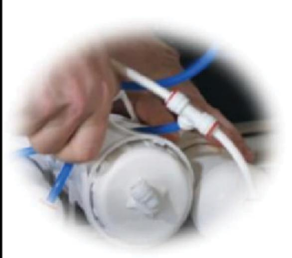
**5. OPEN MEMBRANE HOUSING CAP** - Locate your membrane spanner and open the Membrane Housing. Membrane housing caps can be unscrewed by hand.
