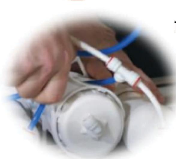
19. TIGHTEN HOUSING, FITTINGS OR CONNECTIONS - If tightening doesn't stop the leak, you may need to replace the faulty component or fitting, or consider using plumber's tape for threaded connections. If this occurs, please contact us.
