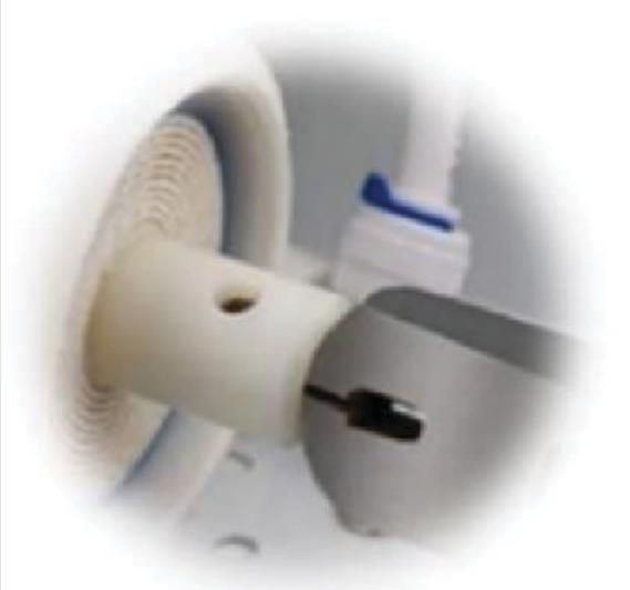
**6. REMOVE MEMBRANE -** Remove the cap from the membrane housing, then by using a pair of needle nose pliers pull out to remove the membrane with a twisting motion and discard the used Membrane.
