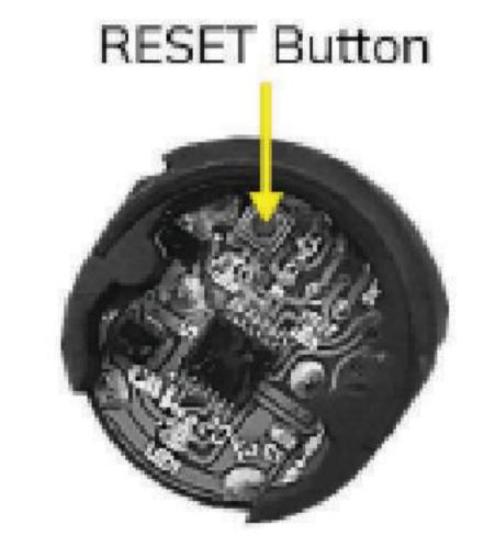
5. Reinstall battery seat assembly into the faucet lever, battery side facing outwards. The slotted end must be oriented toward the faucet.
