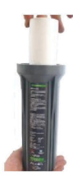
**6. INSTALL NEW CARTRIDGES -** Drop in new filter cartridges into the same housing WITH PACKAGING REMOVED. When installing the new filter cartridges, please double check that the new cartridge and the current cartridge have the same specifications.
