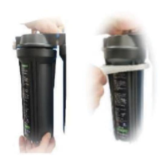
**8. CLOSE THE HOUSINGS -** Screw on housing sump. Tighten the housing using the spanner supplied.
