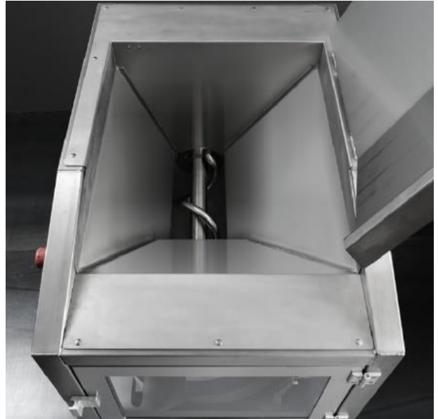
Dough Hopper and Auger
