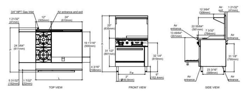
\*Warning: The minimum supply pressure on this appliance must be set at 4 water column inches for natural gas and 10 water column for propane gas. Each unit has a 3/2" gas connect at the rear of the appliance.
