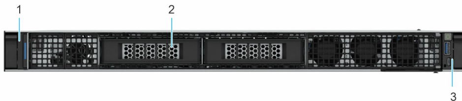
Figure 1. Front view of 2 x 3.5-inch drive system
