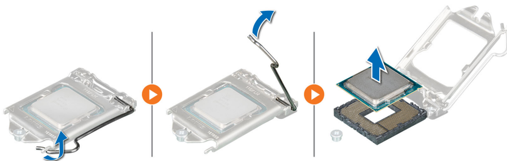
Figure 57. Removing the processor
