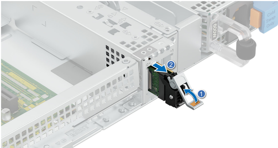
Figure 73. Removing the BOSS-N1 M.2 module
