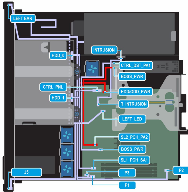
Figure 39. Configuration 0: 2 x 3.5 inch SATA- no Backplane with cable PSU and BOSS-N1 (optional)
