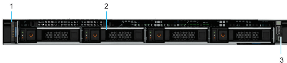
Figure 1. Front view of 4 x 3.5-inch drive system
