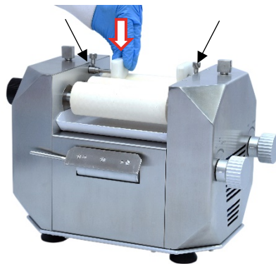
2. Loosen Roller Guide Lock Bolts. Place Roller Guide between center and rear Rollers, flat side up.
