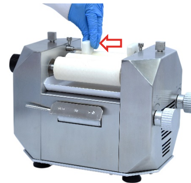
3. Slide Roller Guide into hole. Repeat for second Roller Guide on opposite side.
