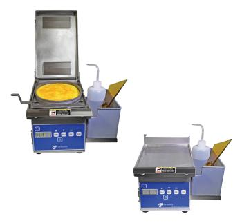
The base unit features an easily interchangeable rack and cover assembly for round eggs or omelets.
