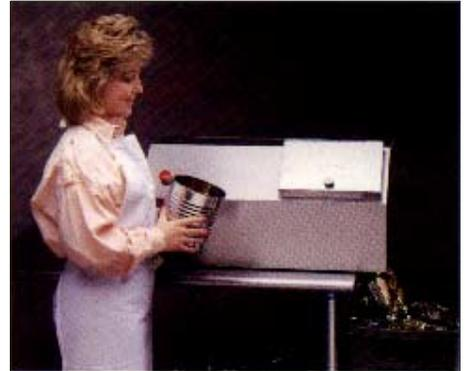
Crushed can falls into receptacle.
