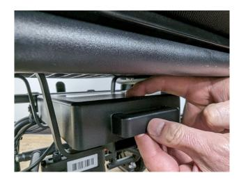
To remove the battery, press the release button and slide the battery towards you.
