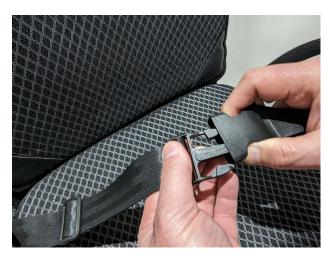
Open the seatbelt by pressing in the two buttons either side.
