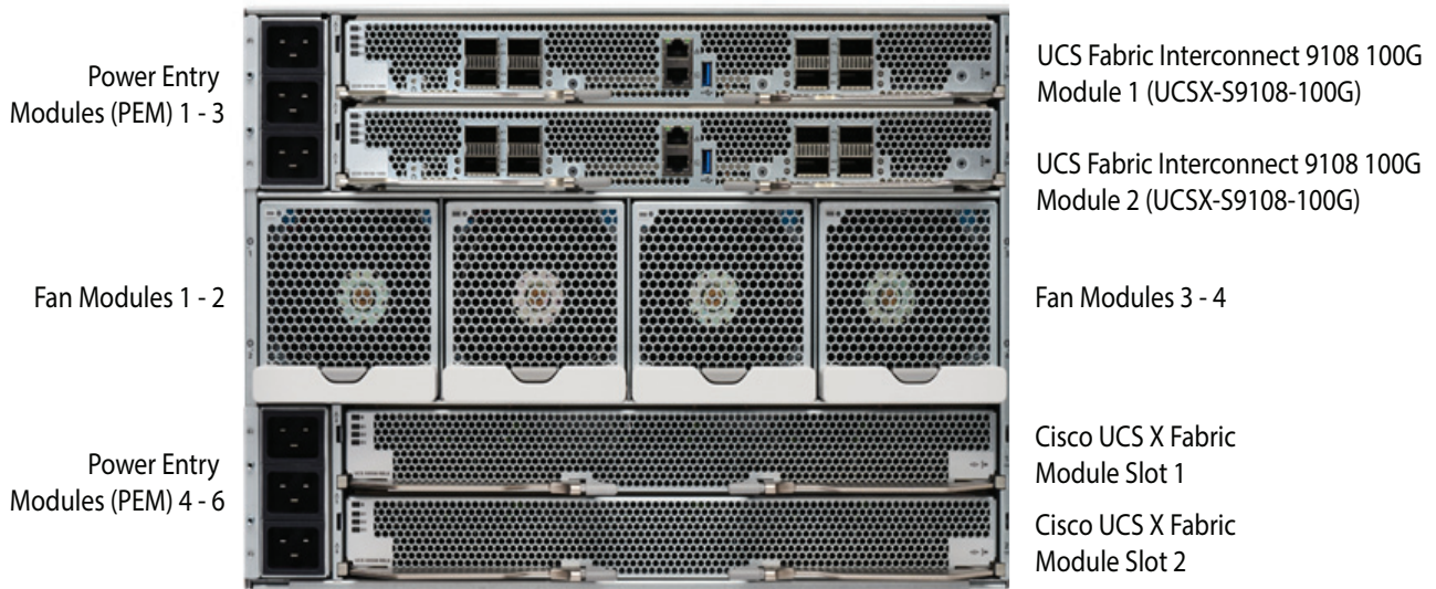
Figure 5 Cisco UCS X9508 X-Series Direct Rear View with UCSX-S9108-100G (top) and 2 Fabric Module Slots (bottom)
