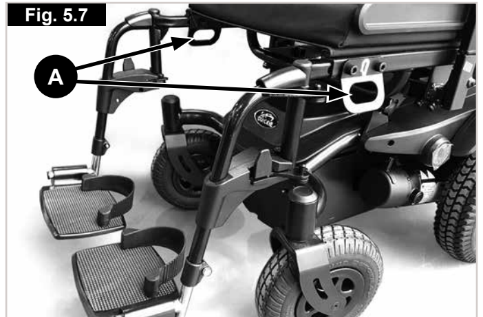
Position of the Front tie down restraint., (Fig.5.7 - A).
