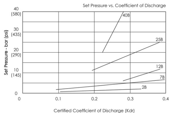
The Kdr value may be used to calculate discharge capacity in accordance with ISO 4126. We recommend contacting us with system details to confirm suitability.
